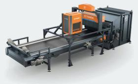
As a complementary solution to AUTOSORT<sup>™</sup>, GAIN<sup>™</sup> deep learning technology utilizes neural networks to differentiate wood chips based on material type. The sorting system effectively separates Wood A from Wood B and recovers MDF from processed wood. It is the ideal solution for creating non-processed wood fractions with **up to 95% purity levels**.
