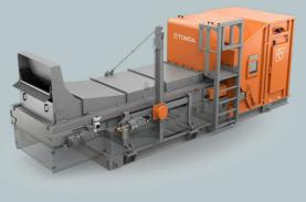
Harnessing the power of x-ray transmission (XRT) technology, X-TRACT<sup>™</sup> measures the atomic density of materials to detect waste wood and remove impurities like inert materials, metals, and glass. With a **capacity of up to 30 metric tons per hour** depending on the material stream, X-TRACT<sup>™</sup> delivers exceptional results in waste wood sorting.
