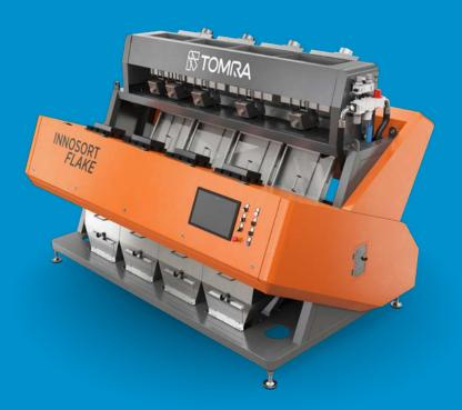
Our new INNOSORT™ *FLAKE* is our most **flexible** color and polymer flake sorting machine. With its powerful combination of sensors and dual-sided full-color cameras, it removes foreign materials and separates flakes by material type, color and transparency. INNOSORT™ *FLAKE* creates high purity flakes ready for extrusion, even from contaminated mixed streams.
