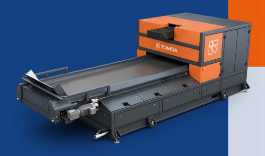
Offering unsurpassed color detection and multi-parameter fraction separation, COMBISENSE™ eliminates most contaminants from even the most challenging ELV, e-scrap and metal waste streams. By allowing granulates to pass through the sorting system twice, high purity levels and a maximum of mono fractions recovery are achieved.
