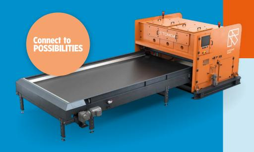
Previously undetectable by NIR sorting technology, black plastics can now be identified and sorted by the AUTOSORT™ *BLACK* plastic sorter. The machine is capable of differentiating between black plastics such as black PE, black PP, black PET and PS without pre-shredding.\* This unit not only fills a gap in waste sorting technology – it creates value. With its high throughput and enhanced resolution, AUTOSORT™ *BLACK* delivers a quick ROI for black plastics.
