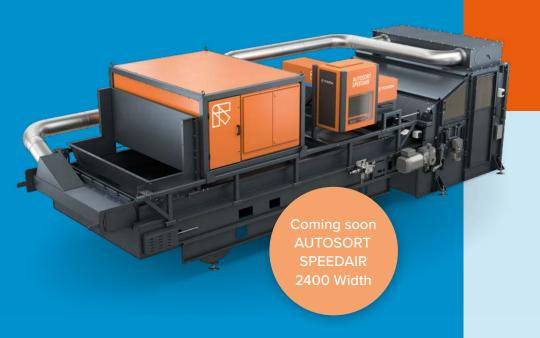
Light materials often don't lie still and are hard to detect when transported on high-speed conveyor belts. With the new AUTOSORT™ SPEEDAIR add-on for AUTOSORT™ machines, fan-driven air inlets generate a steady stream of air above the rapidly moving conveyor belt to stabilize light materials, making it easier to identify fractions. Reducing material movement on a fast-moving conveyor belt moving thus brings higher throughput rates and purity levels.
